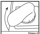
Rotate clockwise to increase cutting depth, counter-clockwise to decrease cutting depth.
